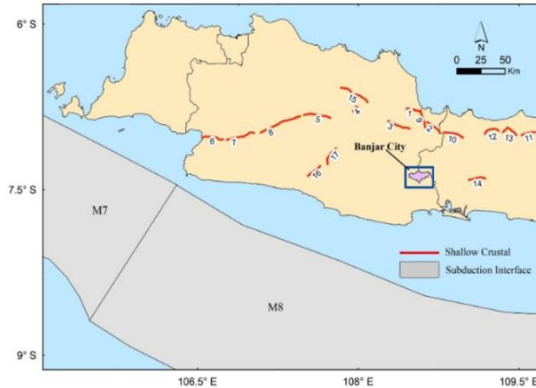
Figure 1. Simplified Traces of The Shallow Crustal Sources are Considered in The Source Modeling
